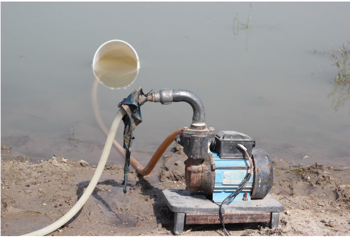
Water motor suck water from pond for drinking purpose.
